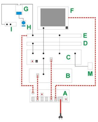
Fig. 7 Cable Connections on the Workstation Models
